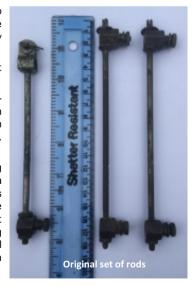
Our throttle linkages are made to the original specifications and will remove play due to wear on the rods and swivel posts. Each linkage has been trial fitted to original Mk1 2.5 Pl Saloon throttle spindles and linkages to ensure correct fit.
