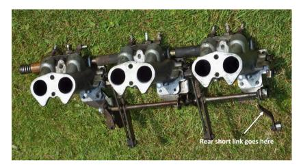
These throttle linkages are manufactured to the same specification as those used on the Lucas Mk 2 petrol injection systems originally fitted to the early mk1 2.5 Pl cars.
