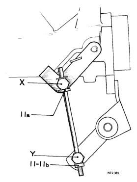
These throttle linkages are made to the original specifications and will remove play due to wear on the rods and swivel posts. Each linkage has been trial fitted to an original CP throttle spindle and linkage to ensure a correct fit.
